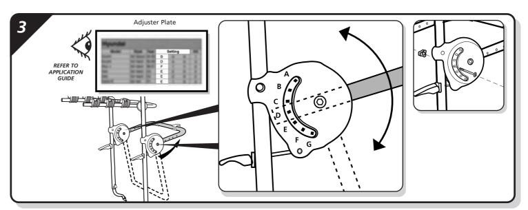
Refer to the enclosed application list to find the correct angle for the vehicle support arm for your car. Insert the bolts from the outside faces in the specified holes A, B, C, D, E, F or G.
